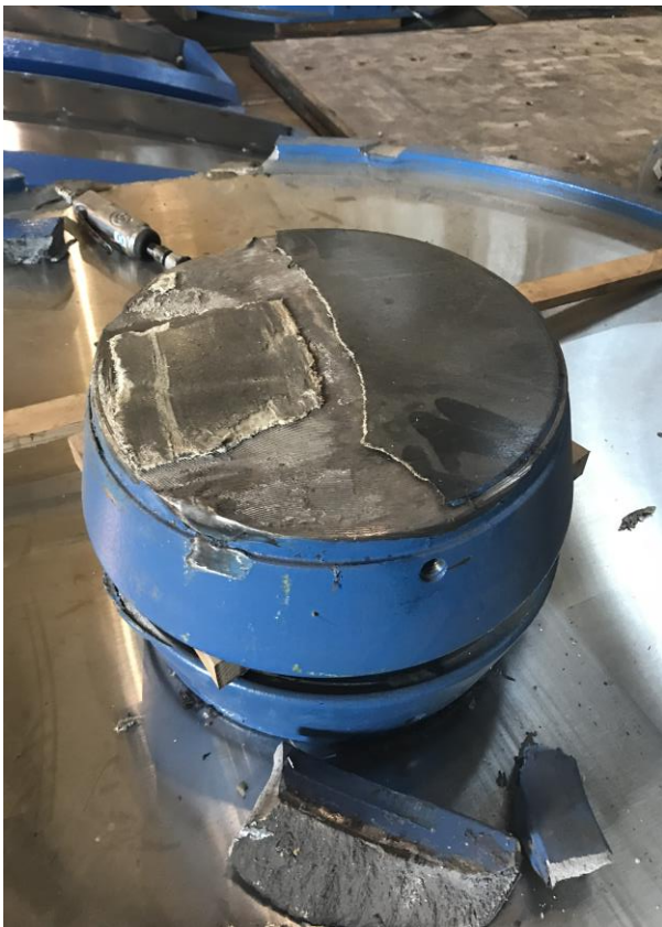
Figure 5: One of the bearing after destructive prototype testing.
