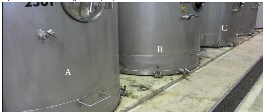
Figure 3: Earthquake related damage data for flat-based wine tanks
