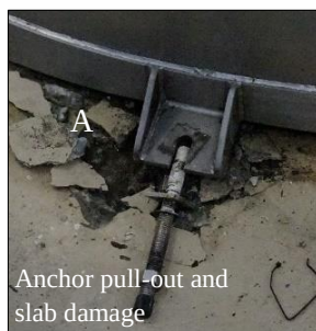
Figure 4: Damaged small capacity (25 kL) flat-based wine tanks
