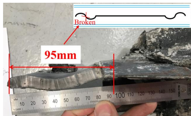
Figure 10: Effective length measurement for BRB specimen
