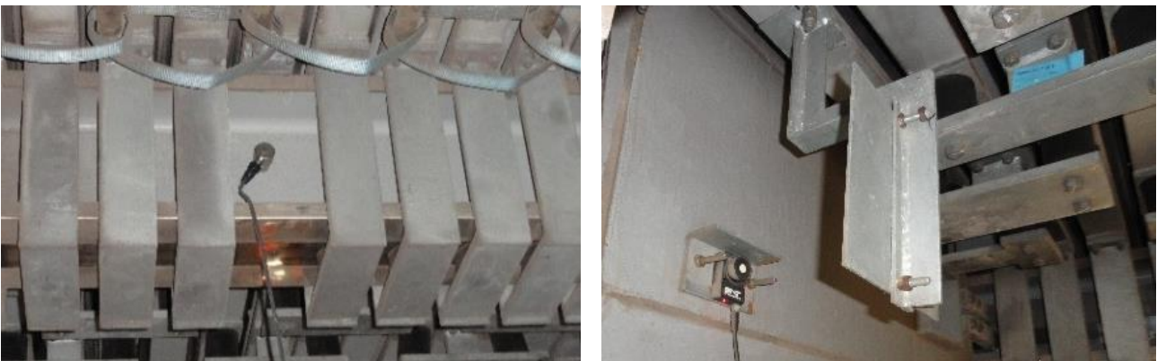
Figure 5: An accelerometer at the location of a temporarily removed stirrup during fault simulation and measurement of resulting vibrations and modal analysis (left) and an ultrasonic displacement sensor (right)
