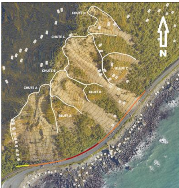
Figure 2: P7 zones and temporary protection. White = zone outlines, yellow = earth bund, orange = double stacked containers, red = single stacked containers
