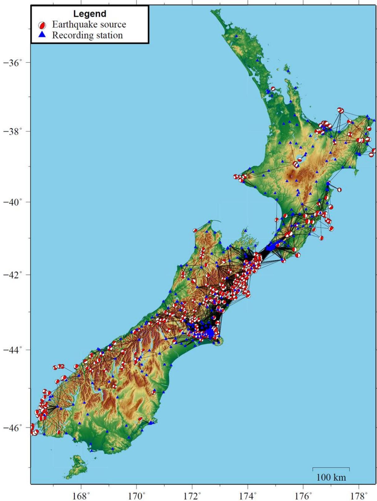
*Figure 1: 609 Earthquake sources and 383 strong motion stations (87 of which do not have high quality records) considered. Schematic ray paths of observed ground motions are also shown as black lines. A total of 5472 ground motions satisfy the quality criteria and are used for simulation validation.*
