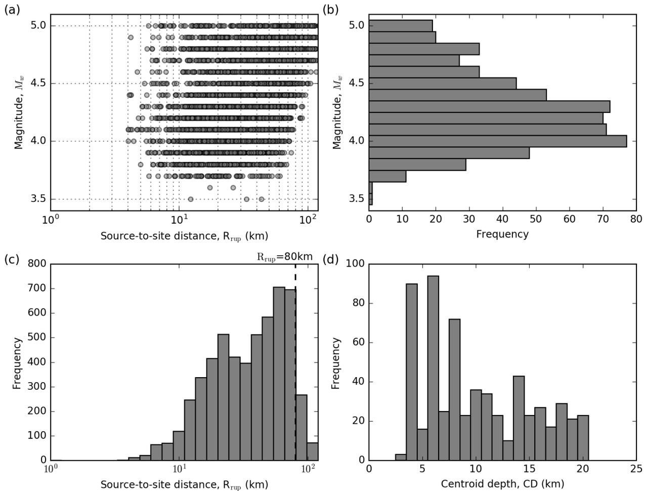
Figure 2: Earthquake source and ground motion distributions: (a) source-to-site distance versus magnitude plot; (b) magnitude distribution; (c) source-to-site distance distribution; (d) centroid depth distribution.
