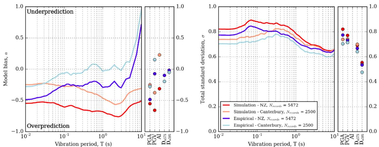
Figure 5: Simulated and empirical prediction for SA as a function of vibration period, and five other IMs: (a) systematic model bias,  $a$ ; and (b) total standard deviations,  $\sigma$ .
