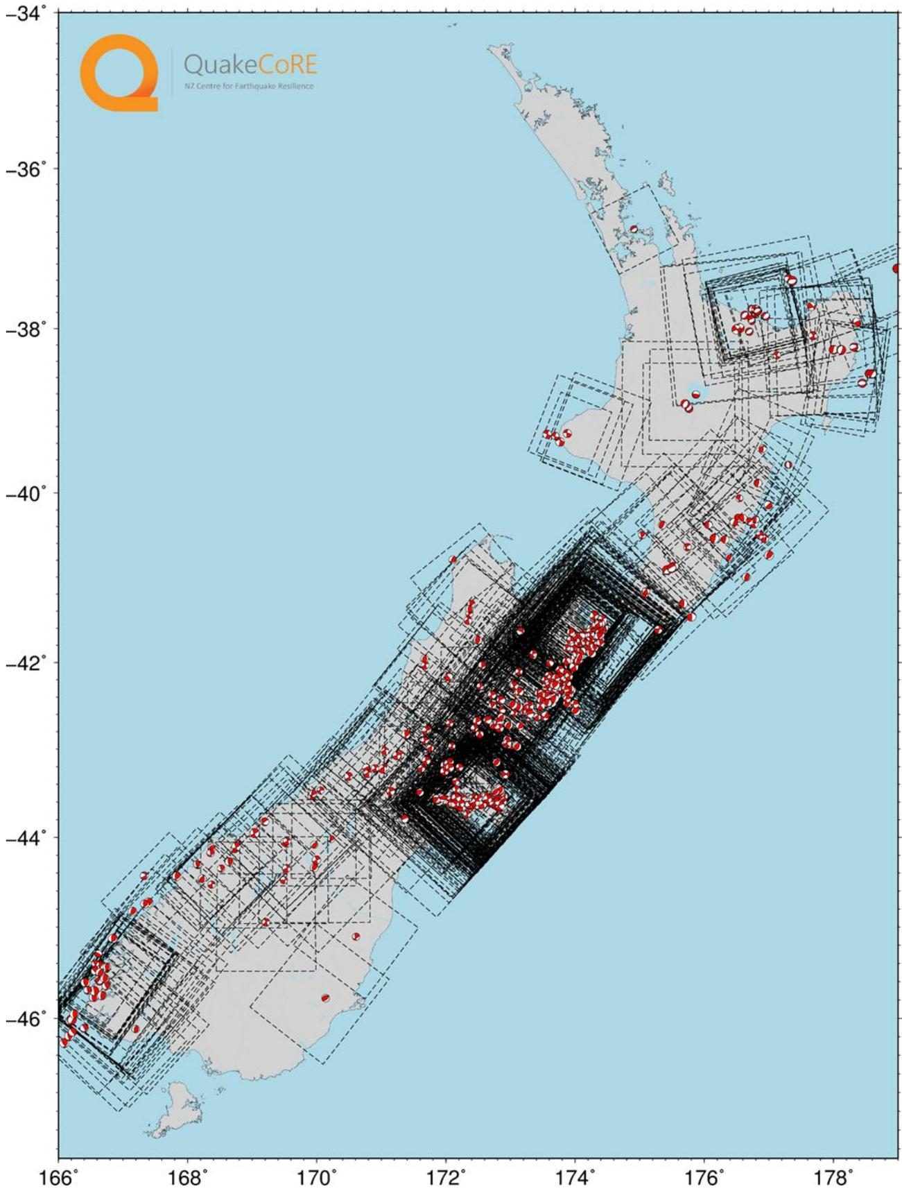
Figure 4: Optimised simulation computational domains for the 609 earthquake events considered.
