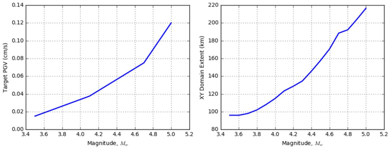
Figure 3: Simulation computational domain size determination: (a) adopted variable PGV threshold as a function of magnitude; and (b) corresponding XY-extents.
