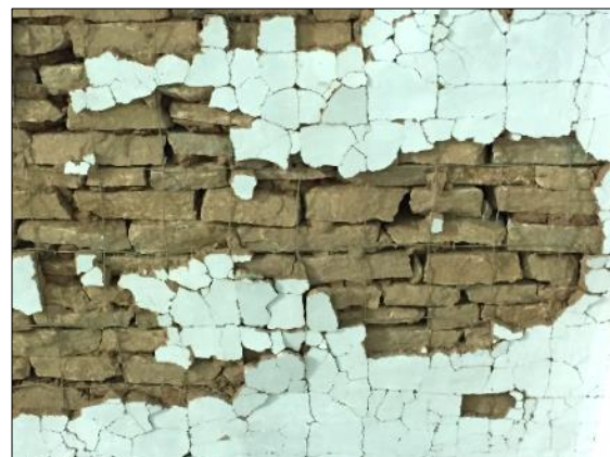
(b) Close-up view of wall, note wide cracks due to sliding of stones, exterior face of 2/3rd model (DT 1)
