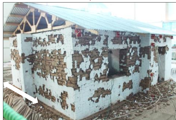
(b) Close-up view of wall, note wide cracks due to sliding of stones, exterior face of 2/3rd model (DT 1)
