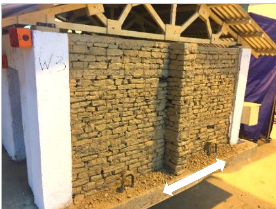
(a) Spalling of plaster and sliding of stones, interior face of 2/3rd scale model (DT 1)
