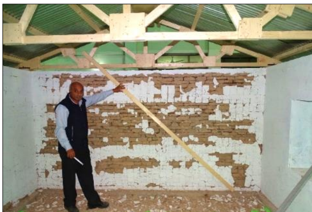
(a) Spalling of plaster and sliding of stones, interior face of 2/3rd scale model (DT 1)
