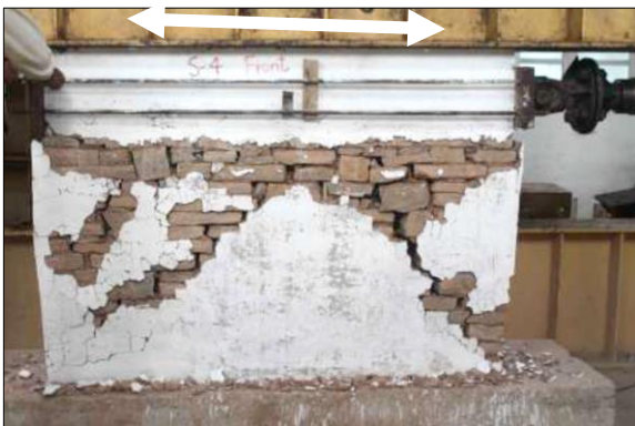
(a) Testing of wall pier without containment mesh under shear
