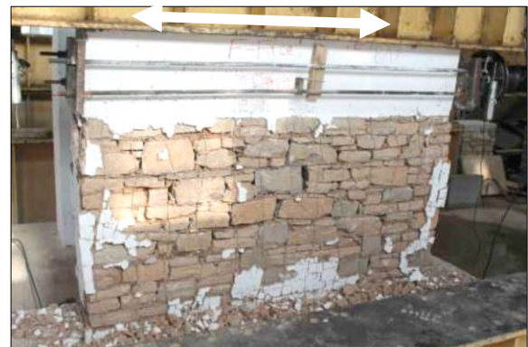
(b) Testing of wall pier with containment mesh under shear
