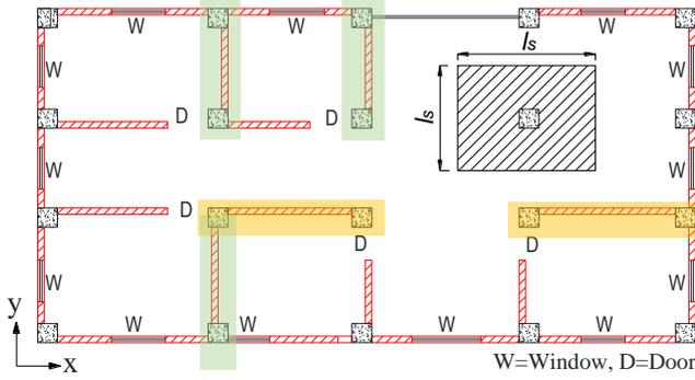
Figure 5: Typical floor plan showing the location of masonry infill
