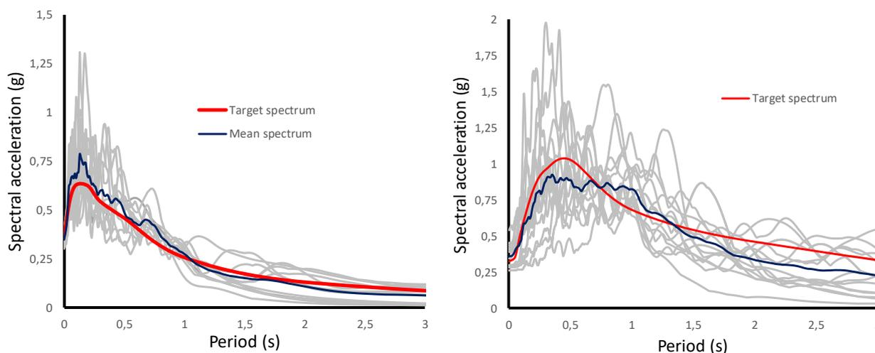
Figure 2: NBCC 2015 design acceleration spectrum, individual record spectra and mean 5% damped elastic acceleration spectrum for calibrated ground motions: (a) MTL-E and (b) VCR-E
