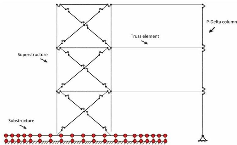
Figure 3: OpenSEES model of structure-foundation-soil system (adapted from Aguero (2006) and Prishati (2008))
