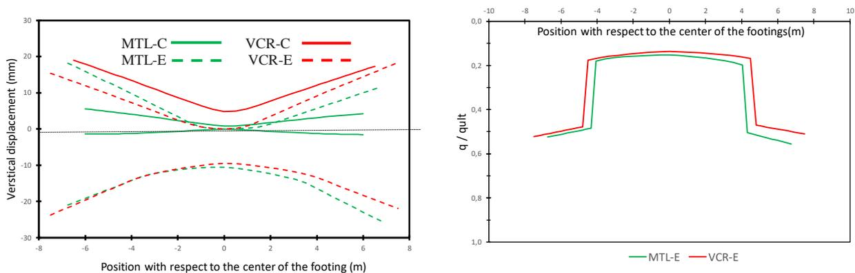
Figure 4: (a) Permanent soil settlements, foundation uplifts and (b) normalised forces in the springs
