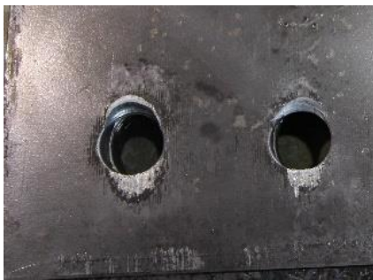
Figure 14: Abrasion and splitting of hole edges in filler plates
