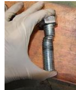
Figure 16: Deformation of bolt at failure
