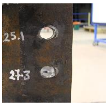
Figure 10: Damage in flange splice plate Figure 11: Elongation of holes in web
