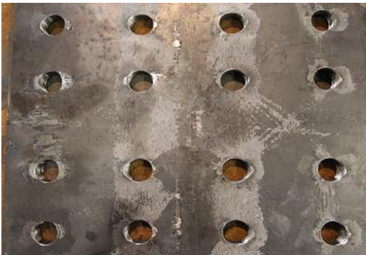
Figure 10: Damage in flange splice plate Figure 11: Elongation of holes in web
