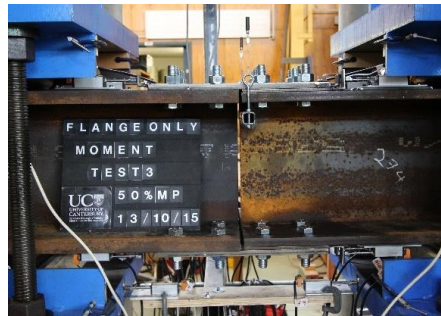
Figure 15: Elongation at splice joint
