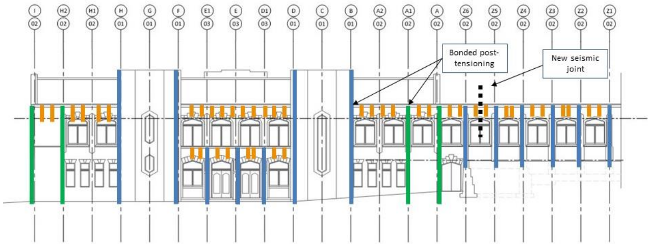
Figure 6: Strengthening with post-tensioned bars on the Southwest elevation
