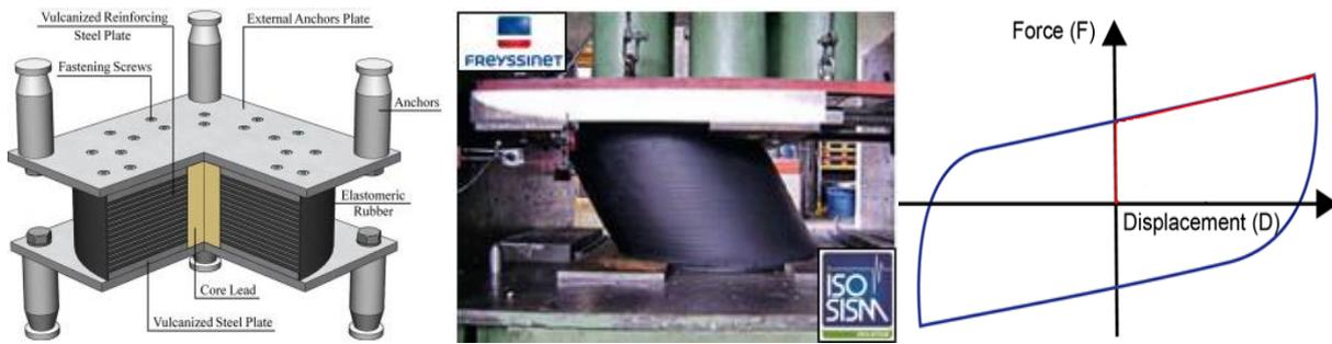
Figure 3: LRB geometry (left), horizontal flexibility (centre) and hysteretic shear behaviour (right)
