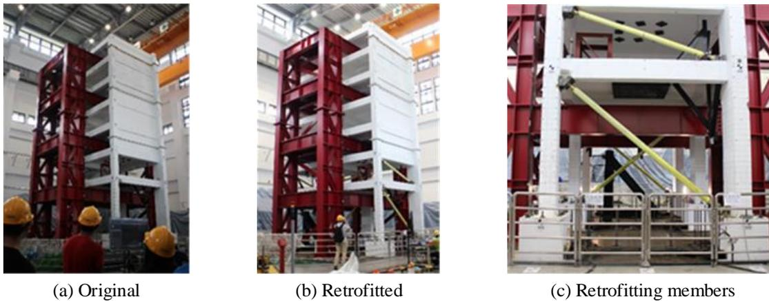
Figure 5: The retrofitted and original specimen.
