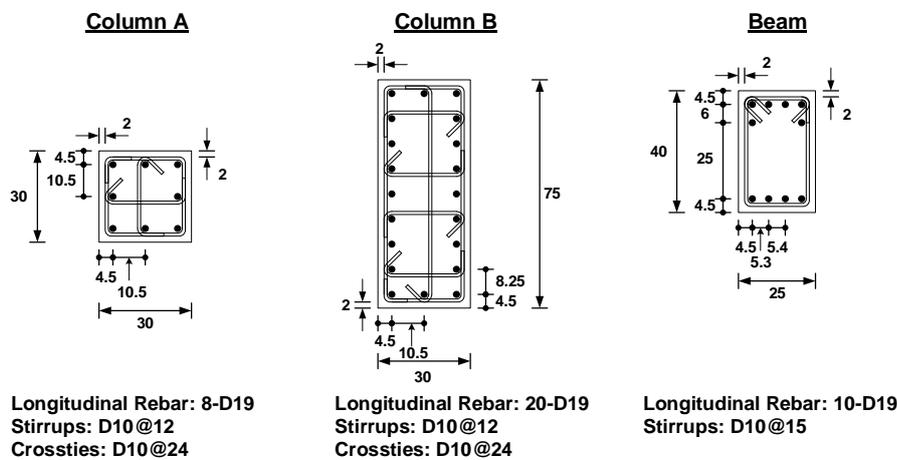
Figure 4: The information of cross-section (unit in cm)
