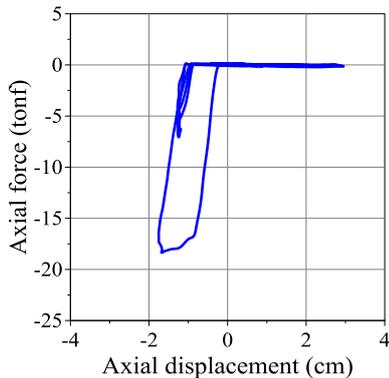
Figure 8: The energy dissipation of brace at 2<sup>nd</sup> story
