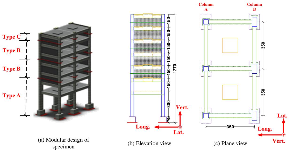
Figure 3: The dimension of the specimen (unit in cm)
