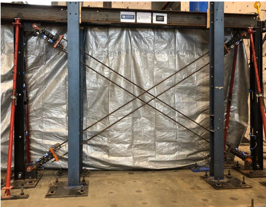
Figure 6: Full test setup including the main and protection frames
