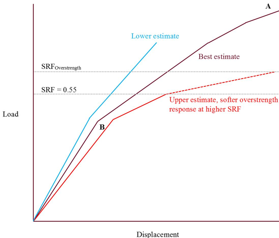
Figure 2: Example load displacement plot with lower, best and upper estimate behaviour indicated. Note that upper estimate stiffness has a softer response to account for the greater uncertainties present at the higher SRF. Point A describes the displacement to mobilise the geotechnical ultimate capacity (as outlined in Module 4). The change in stiffness at point B is due to the pile mobilising the full shaft resistance
