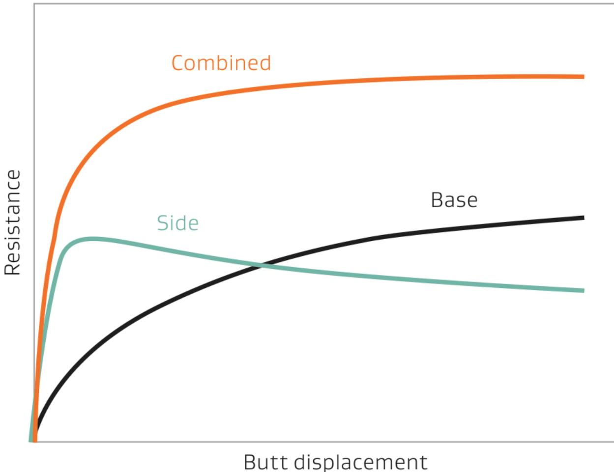
Figure 1: General load-displacement response of a piled foundation. (Reproduced from NZGS/MBIE Module 4, 2016)
