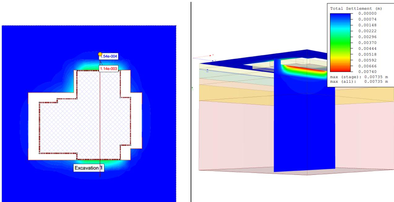
Figure 3: Settle 3D model showing the excavation stage
