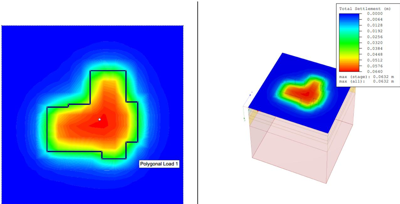
Figure 4: The modelled Terefil raft combined with building loads
