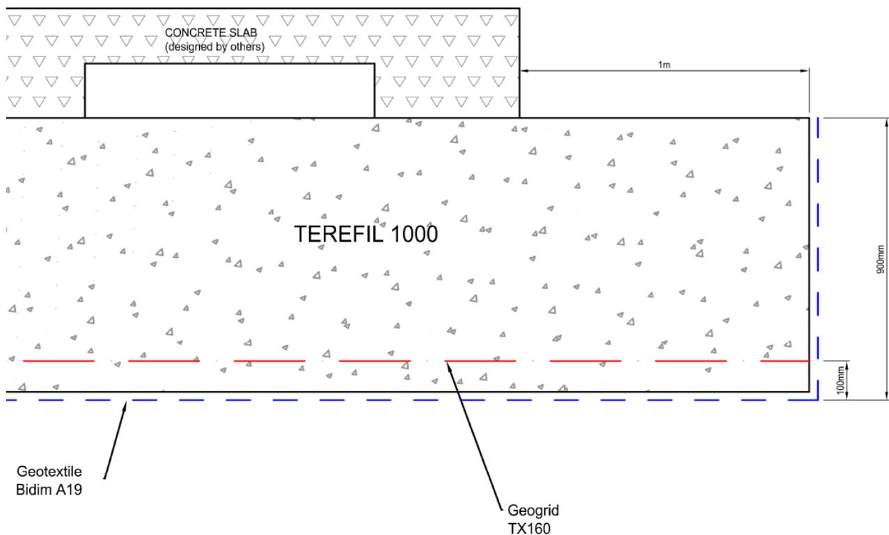
Figure 1: Schematic cross-section of a Terefil raft design
