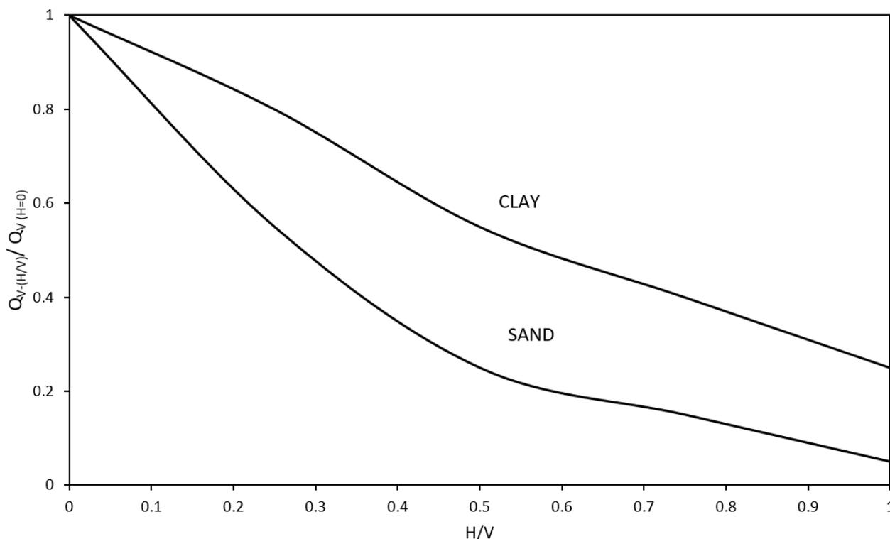
Figure 2: An example of effect of horizontal loading on vertical bearing capacity (Based on Hansen, 1970)
