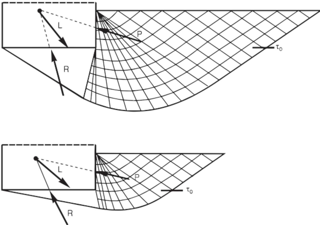
Figure 1: Rupture surfaces of inclined footing loads. (Source: Hansen 1970)
