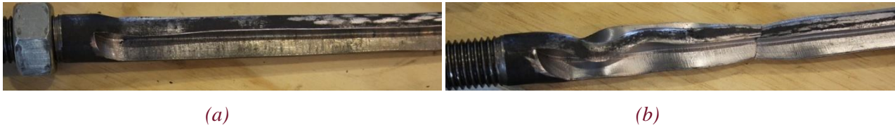
Figure 5: Snake-shape local buckling and fracture of grooved dissipaters (a) GD-1, (b) GD-2
