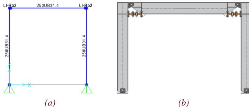
Figure 10: (a) SAP2000 model (b) Position of RSFJ in MRF
