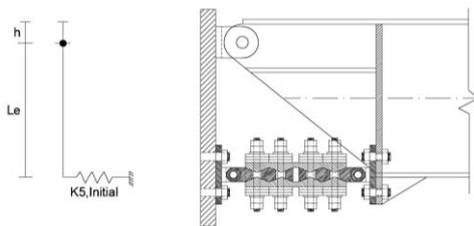
$$M_{slip} = F_{slip} \times L_e = (K_{initial} \times L_e \times \theta_{slip}) \times L_e = (K_{initial} \times L_e^2) \times \theta_{slip} = K_{\theta-initial} \times \theta_{slip} \quad (3)$$
