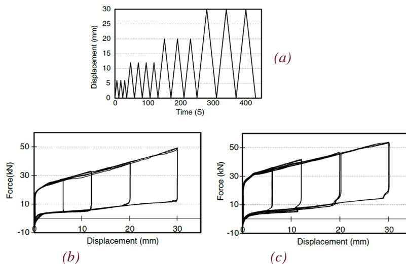
*Figure 6: RSFJ component test results (Hashemi et al. 2017): a) The applied displacement schedule b) Hysteretic behaviour for  $F_{slip} = 24$  kN c) Hysteretic behaviour for  $F_{slip} = 31$  kN*
