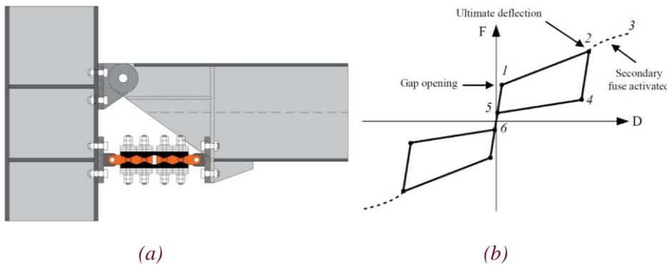
Figure 4: The concept of self-centring MRF with RSFJ: (a) general arrangement (b) theoretical hysteresis
