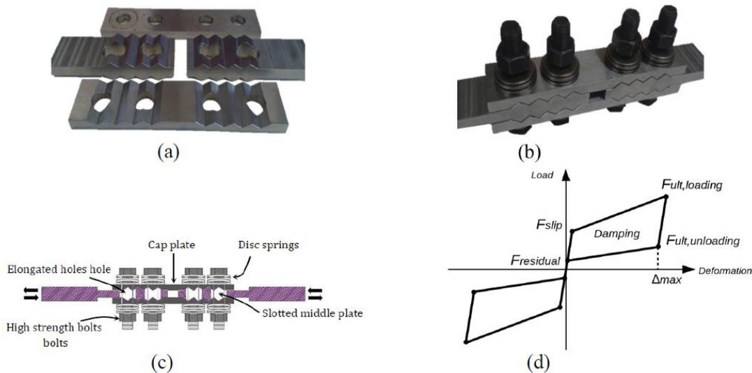
Figure 3: RSFJ: (a) sliding plates (b) assembly (c) components (d) hysteresis
