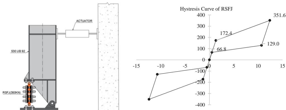
Figure 12: (a) MRF test setup with RSFJ (b) predicted hysteresis curve of RSFJ
