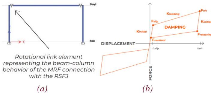
Figure 9: (a) SAP2000 modelling (b) Design parameters
