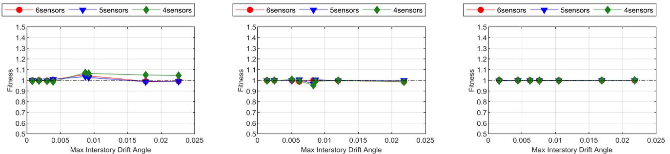
Figure 4: Accuracy of PWCPI for 28-story building during the (a) 1940 Imperial Valley earthquake, (b) 1995 Kobe earthquake, and (c) 1994 Northridge earthquake
