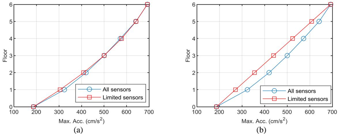
Figure 7: Height-wise distribution of maximum acceleration using the PWCPI procedure: (a) three sensors; (b) two sensors
