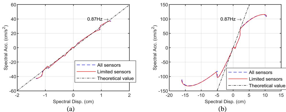
Figure 1: Comparison of capacity curve from THA and PWCPI: (a) linear case; (b) nonlinear case
