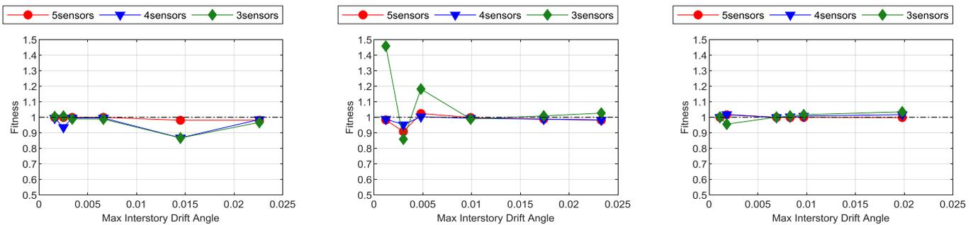
Figure 3: Accuracy of PWCPI for 18-story building during the (a) 1940 Imperial Valley earthquake, (b) 1995 Kobe earthquake, and (c) 1994 Northridge earthquake
