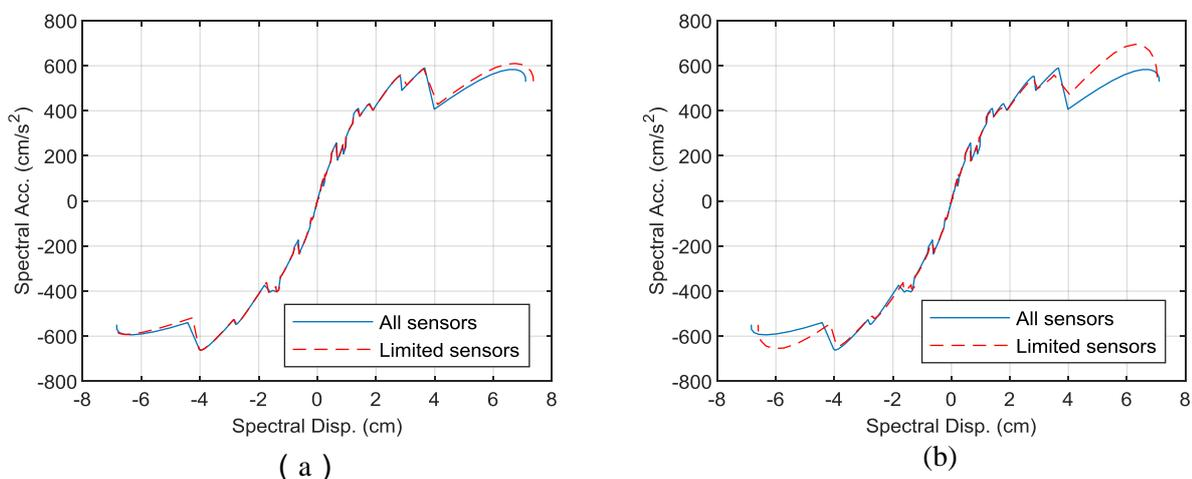
Figure 6: Capacity curve of six-story building: (a) three sensors; (b) two sensors
