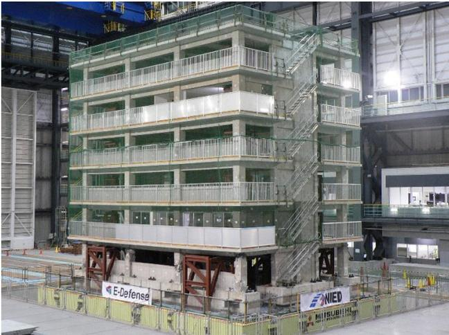
Figure 5: Six-story RC shear wall building test model
