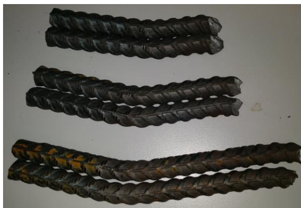
(b) Fractured reinforcing bars
