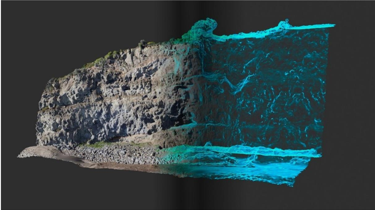
Figure 2 – 3D models assist us in understanding complex geometry and terrain (in this instance the images were captured by laser scanning and unmanned aerial vehicle photography)
