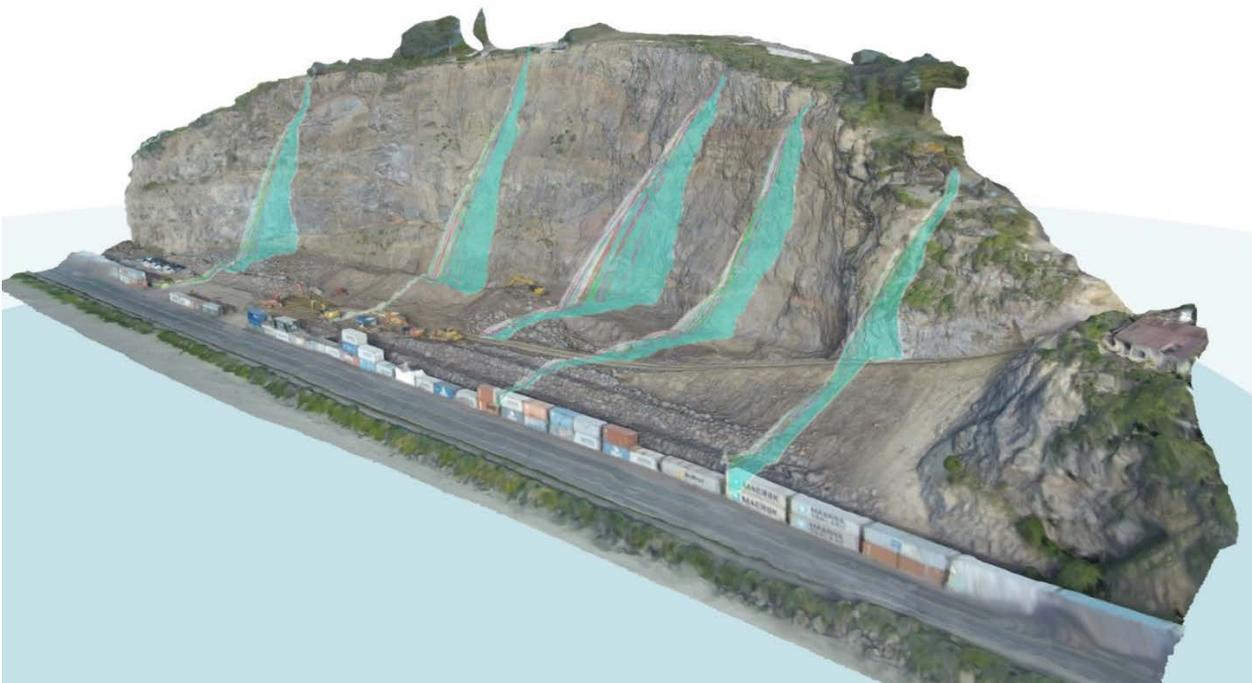
Figure 7 - 3D model with sectional rockfall analysis overlain showing areas where rockfall hazard extends over site traffic corridors
