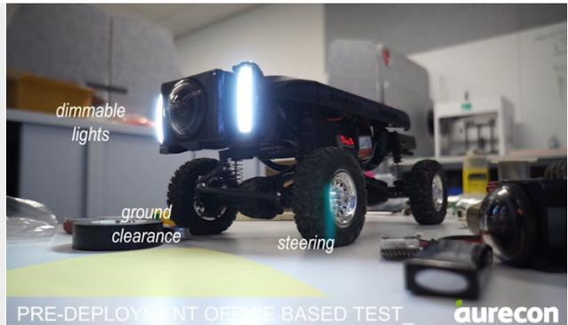
b) final assembly and pre-deployment testing
