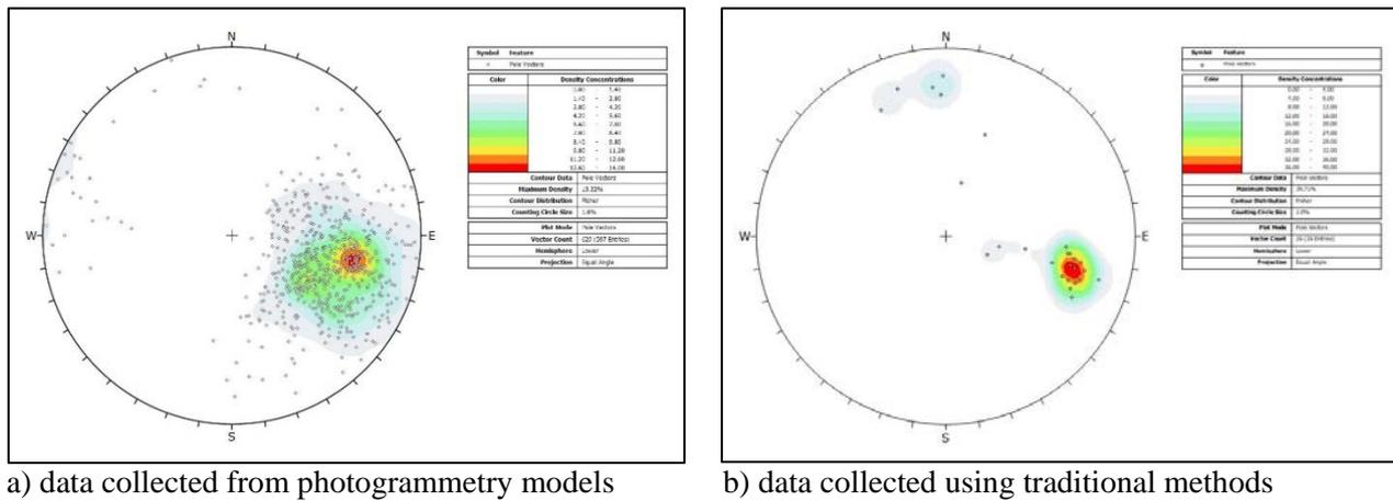
Figure 7 – Comparison of the rock joint data gathered from the photogrammetry model (a) compared with minimal verification data collected on site using traditional methods (b).
