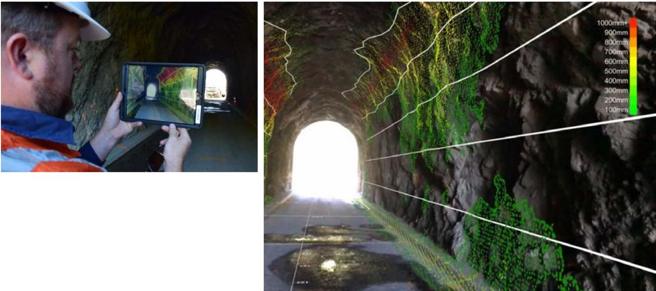
Figure 5 – Augmented reality in use to determine tunnel improvement requirements
