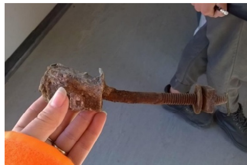
Figure 16: Bottom plate to foundation 'chemical' anchor system.
