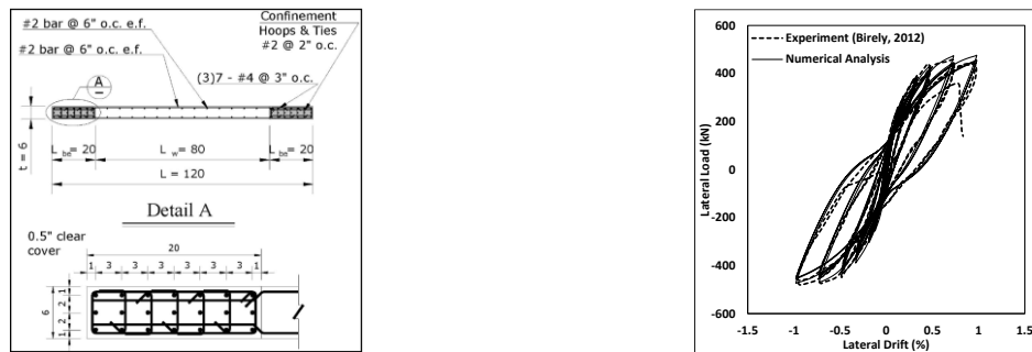
(a) Shear wall layout (Birely 2012)
