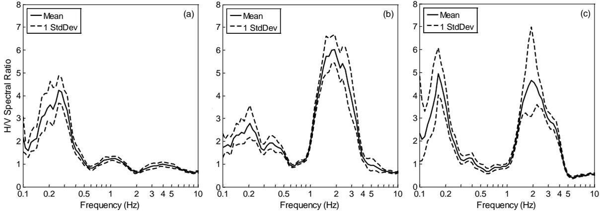
**Figure 3. Example H/V spectral ratio data from ambient noise records across Canterbury (a) Single predominant peak corresponding to deep site period above basement rock, (b) single predominant peak corresponding to shallow site period above gravels, (c) Double peak corresponding to both shallow and deep site periods.**
