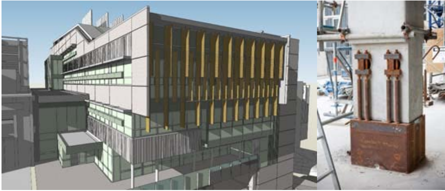
Figure 1. The Alan MacDiarmid building, Victoria University of Wellington (left), and close up of the EMD (right) (BBR Contech 2011).
