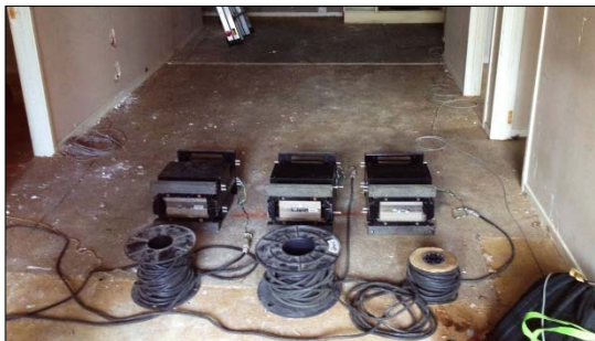
(a) Electro-dynamic shakers set up for testing in the N-S direction
