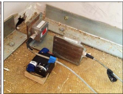
(b) Two types of accelerometers used - standalone (left) and wired (right)
