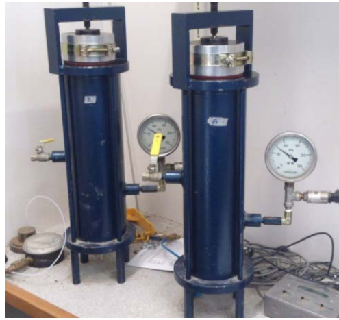
Figure 3. Oxygen permeability test apparatus.
