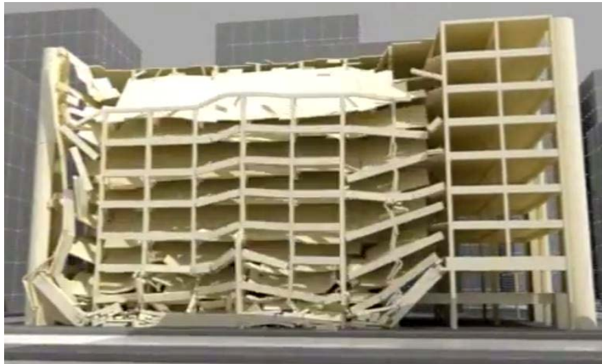
Figure 3. AP Murrah Building Progressive Collapse.
