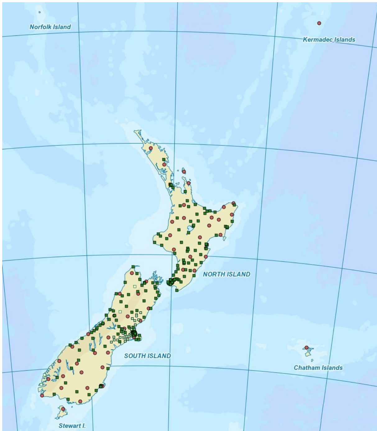
Figure 1. The New Zealand strong ground motion sites. Green symbols are National Strong Ground Motion Network sites and red symbols are National Seismograph Network sites.
