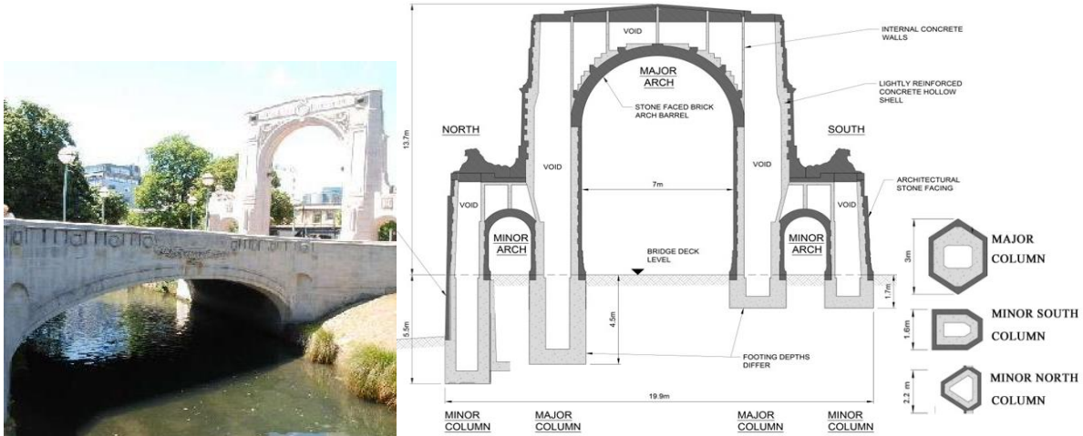
Figure 2. a) The Bridge of Remembrance and the Triumphal arch. b) Drawings of the main sections of the Triumphal Arch. Courtesy of SCIRT.
