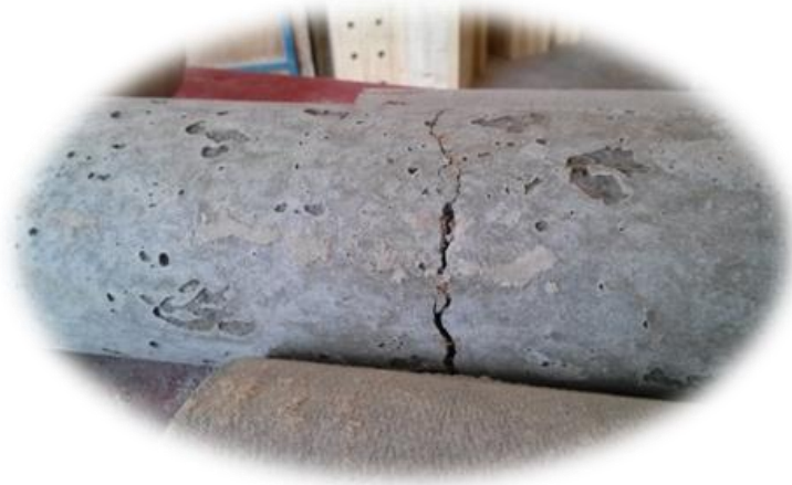
Figure 5. CFRC core after removed the outer FFRP tube
