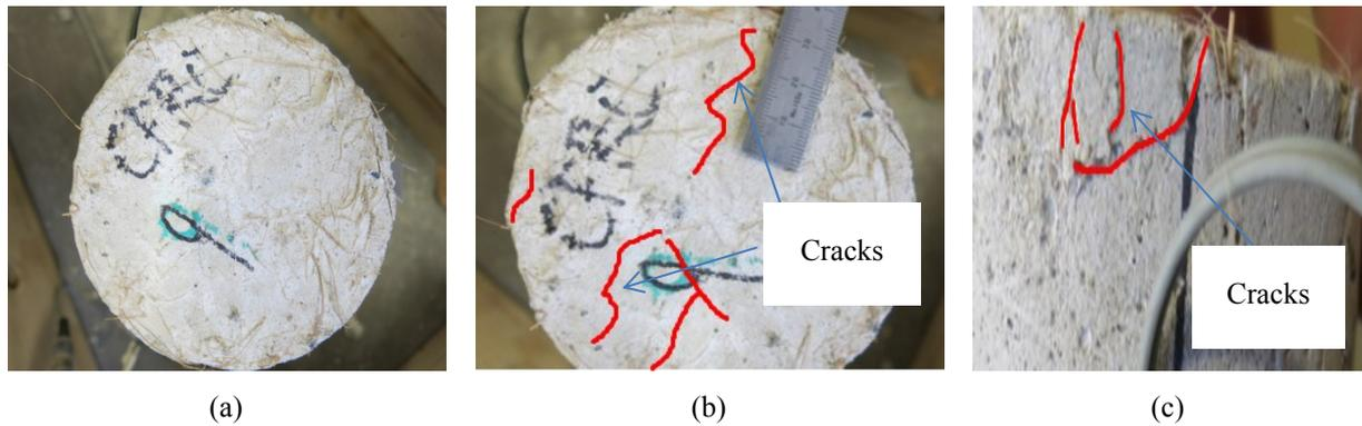
**Figure 7. Influence of coconut fibre on the fibre-concrete composite behaviour: (a) Before impact and after impact (b) top view (c) side view**
