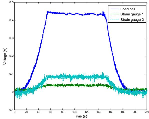
(b) Voltage recorded by the load cell and strain gauges
