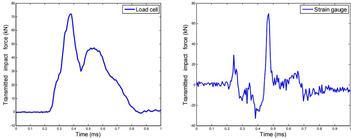
**Figure 3. Force transmitted by plain concrete**
