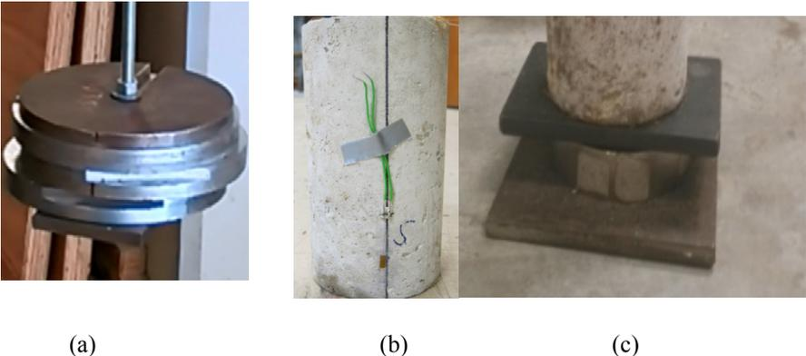
Figure 1. Impact test set up: (a) Drop weight; (b) strain gauge and (c) load cell
