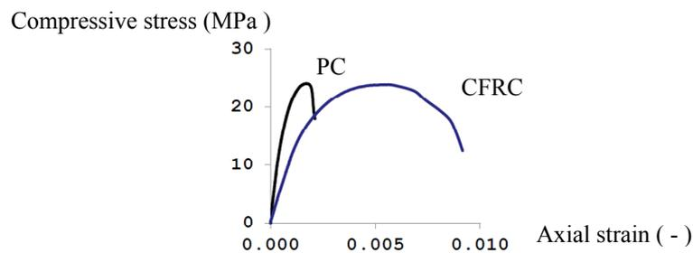
**Figure 5. Influence of coconut fibre on the stress-strain relationship (Yan and Chouw, in print)**
