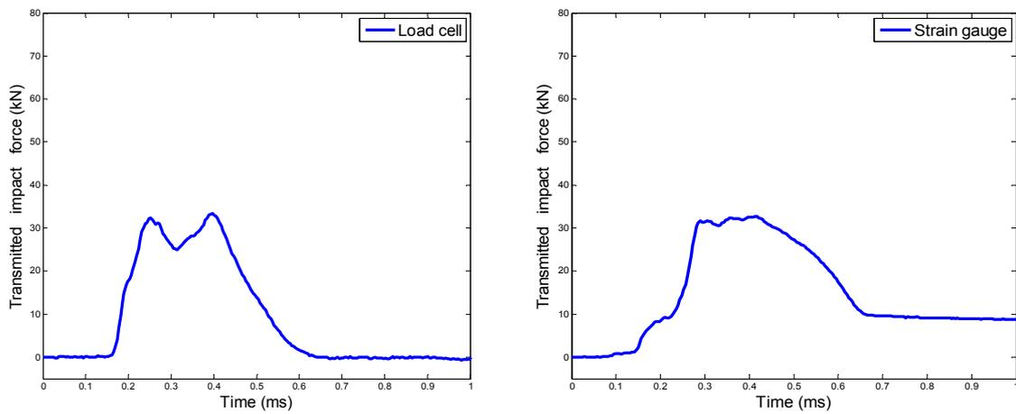
**Figure 4. Force transmitted by CFRC**
