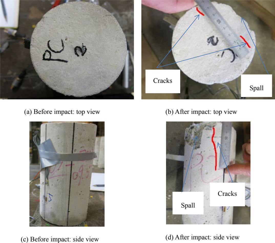
**Figure 6. Views of plain concrete before and after impacting**
