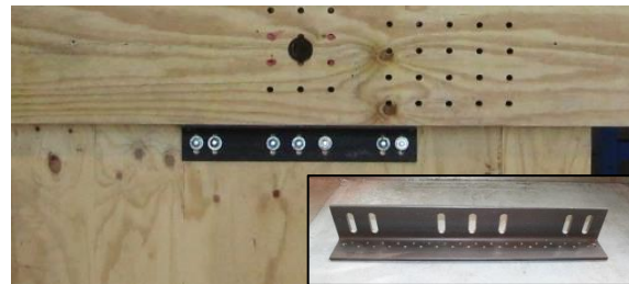
6) steel comb with slotted holes
