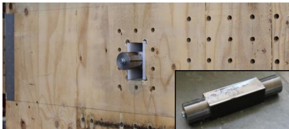
5) centred 65 mm diameter pin with slot in wall
