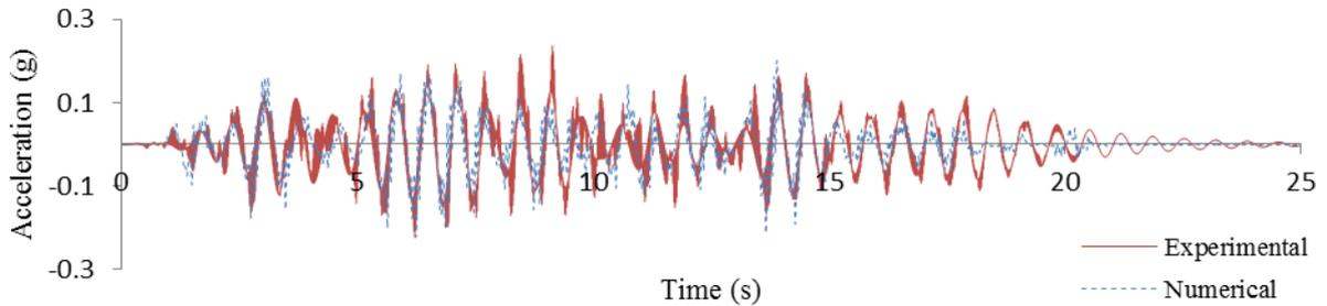
Figure 3. Acceleration at the top of the secondary structure
