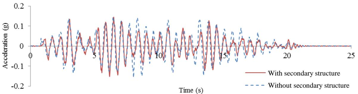
Figure 4. Acceleration at the top of the main structure measured in experiments
