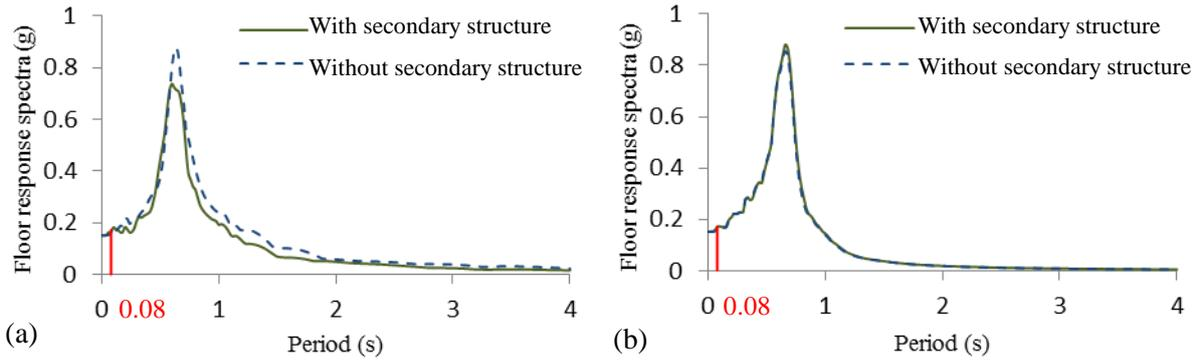
**Figure 6. Floor response spectra from (a) experimental data and (b) numerical prediction**
