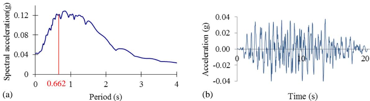
**Figure 2. Ground motion characteristics, (a) response spectrum (b) ground acceleration time history**
