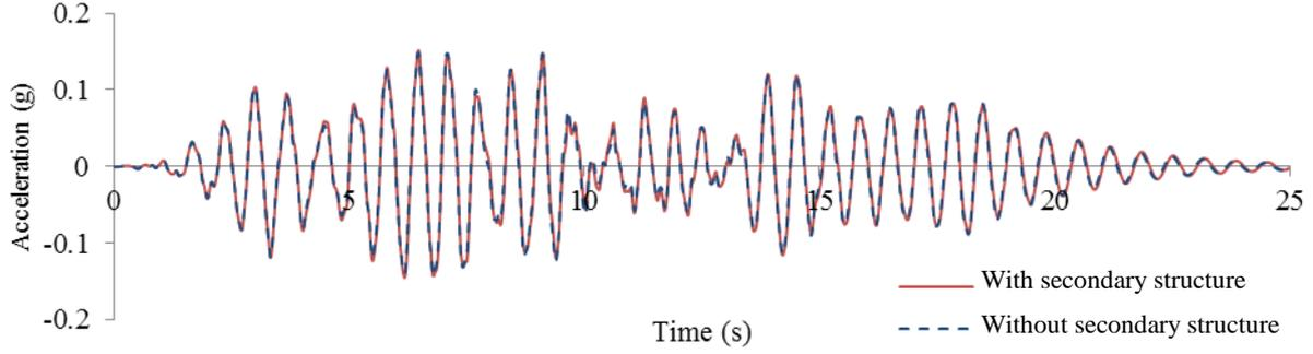
**Figure 5. Acceleration at the top of the main structure obtained from numerical analysis**
