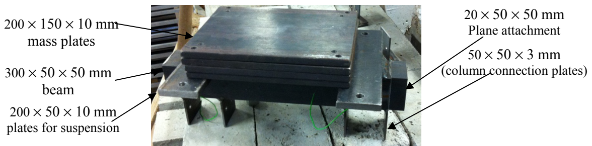
Figure 3. Steel beam constructed for the impact tests
