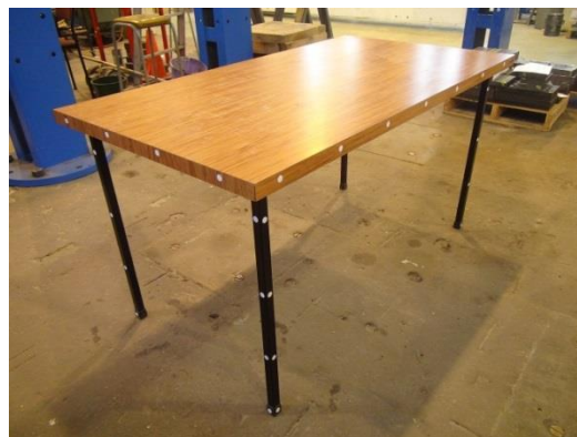
Figure 2. Desks with rubber soles used in shake table experiment
