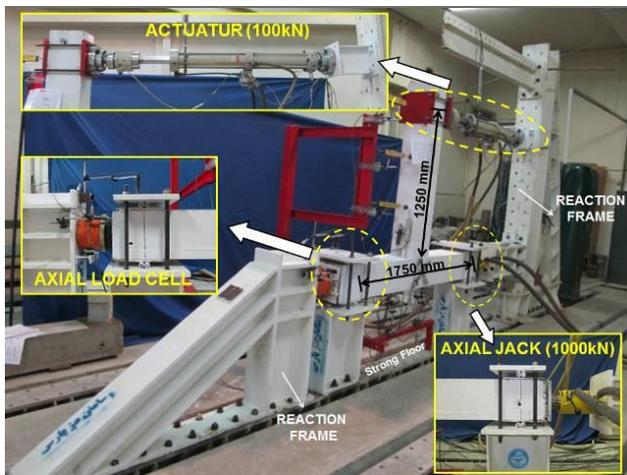
**Figure 2.** View of test setup.
