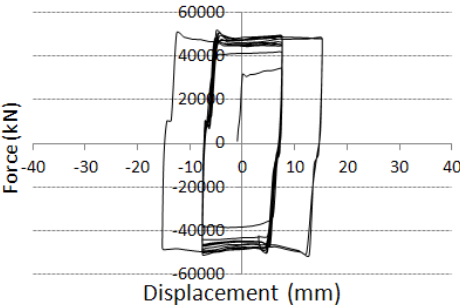
Figure 7. Initial displacement cycles showing build up to peak load.
