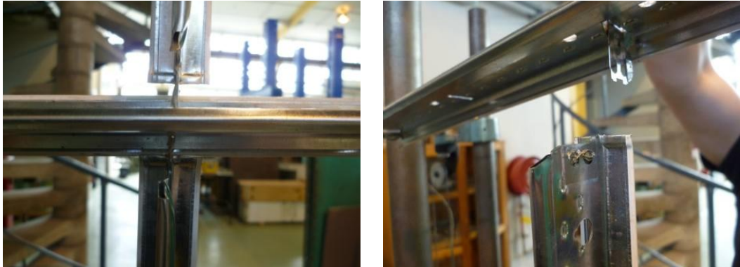
Figure 5. Failure mode of connection in the tensile test (left); Failure mode of the riveted connection (right).
