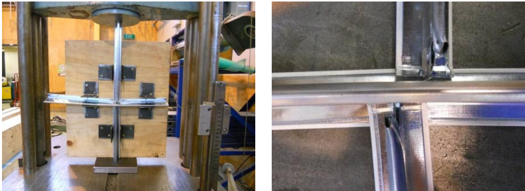
Figure 6. Failure mode in a compression connection specimen
