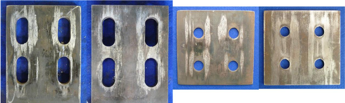
Figure 5: Left to right: surface conditions for cleat with G300 shims, cleat with G400 shims, G300 shim and G400 shim
