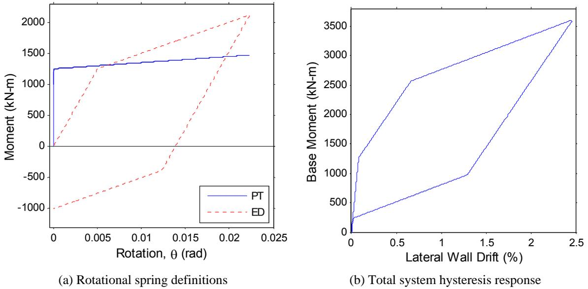
Figure 4 – Two spring lumped plasticity model with idealised hysteresis and unbalanced moment resistance
