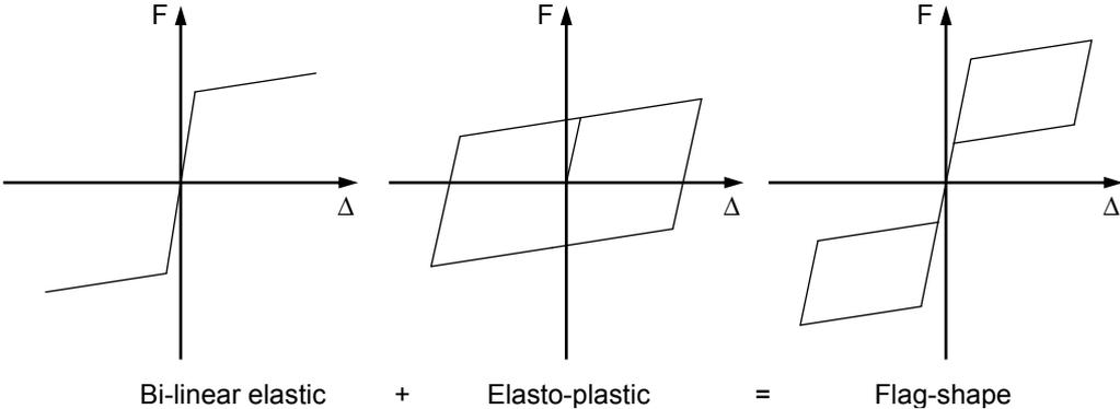
Figure 1 – Idealised flag-shape hysteresis response typically assumed for self-centering systems
