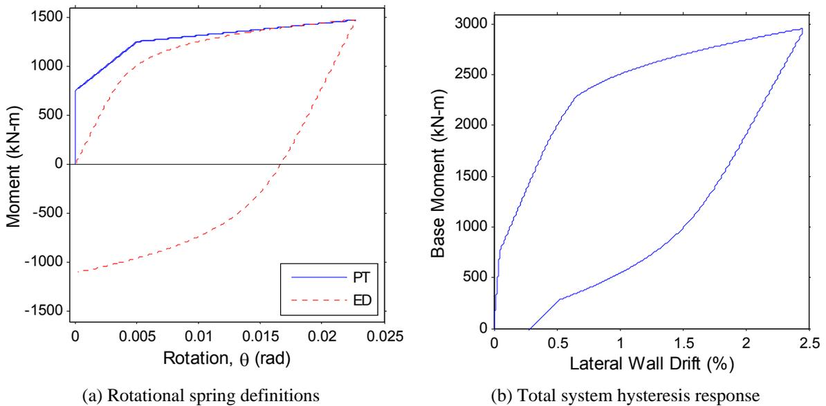
Figure 5 – Two spring lumped plasticity model with realistic hysteresis and equal moment resistance
