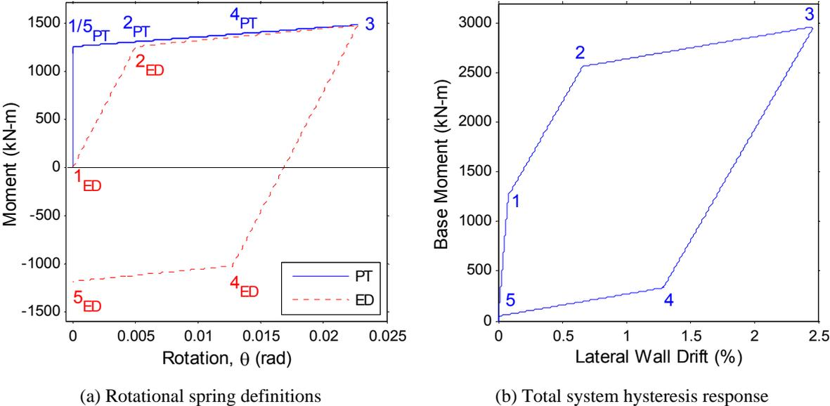
Figure 3 – Two spring lumped plasticity model with idealised hysteresis and equal moment resistance
