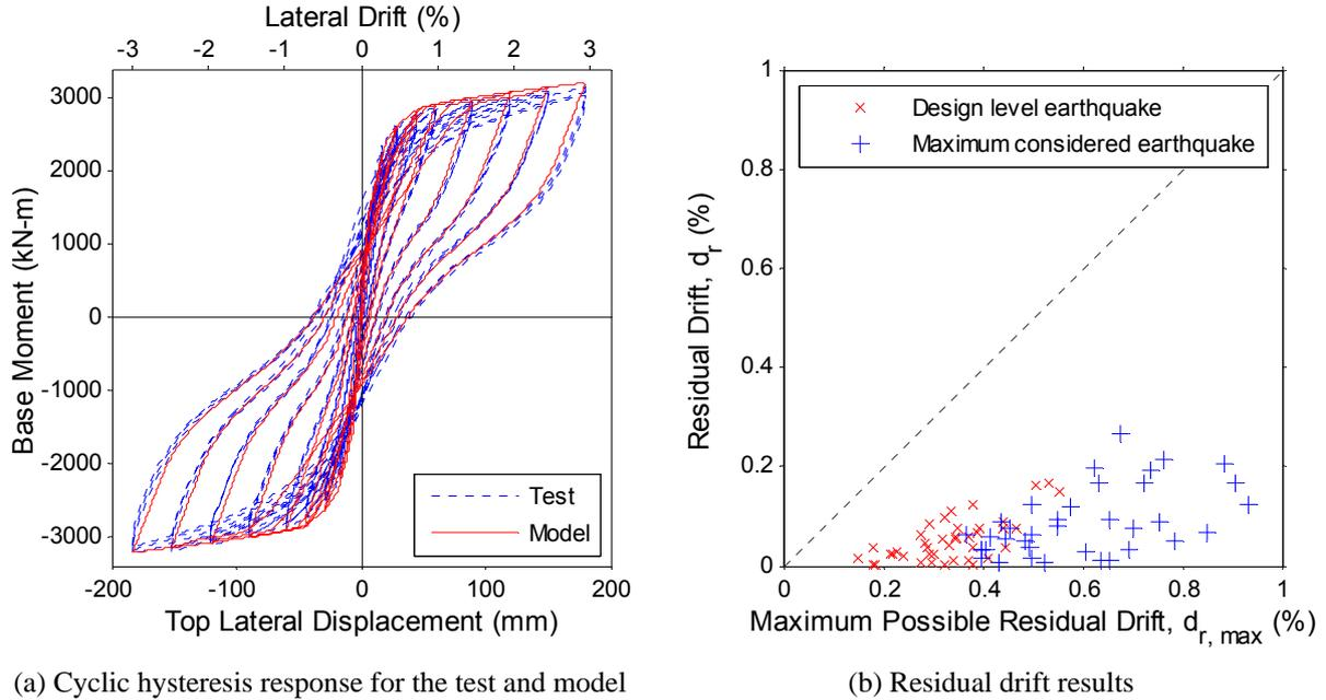
Figure 6 – Time-history analysis of lumped mass models with PreWEC hysteresis response
