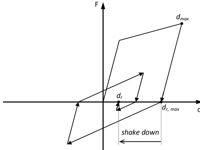
Figure 2 – An illustration of dynamic shake-down behaviour expected for seismic load resisting systems
