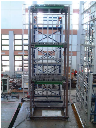
Figure 5 Photo of the shaking table test building in NCREE
