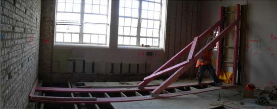
**Figure 4: Out-of-plane test setup**
