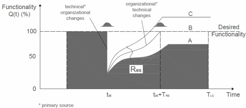
**Figure 1 Schematic representation of seismic resilience**
