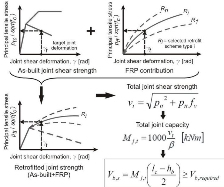
**Figure 2:** Conceptual deformation based design procedure
