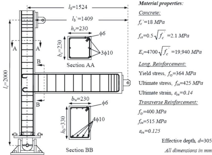
**Figure 3:** Details of analyzed specimen
