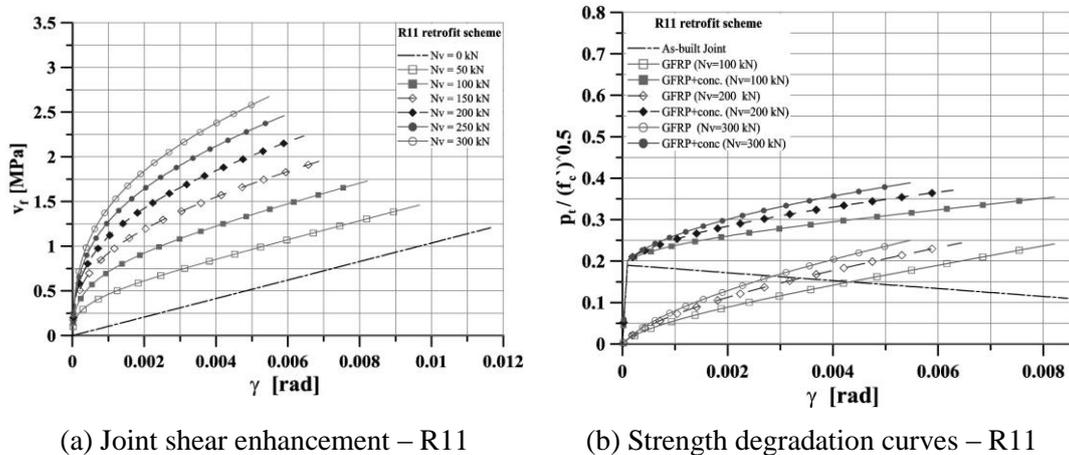
Figure 5: GFRP effect on the behaviour of strengthened joint under varying axial load (cont'd)
