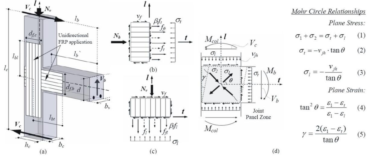
**Figure 1:** Exterior RC joint strengthened with FRP: (a) design dimensions; (b) horizontal force equilibrium; (c) vertical force equilibrium (modified after Antonopoulos et al.); (d) kinematics of as-built joint and Mohr circle definition of plane strain and stress
