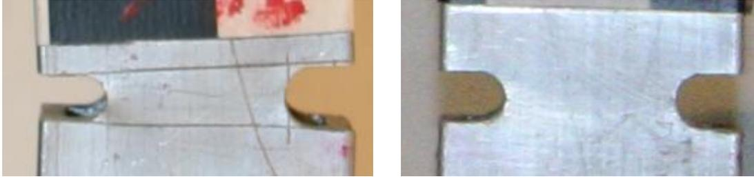
Figure 8: The notched area of the medium (left) and small (right) columns post testing.
