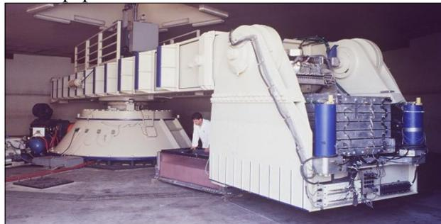
Figure 2: Centrifuge facilities of the University of California, Davis.
