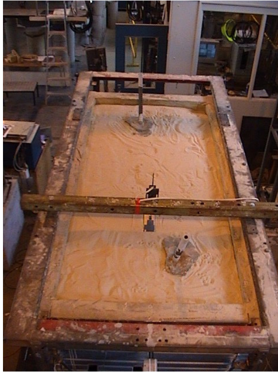
Figure 8. Completed installation of two inclined micropiles.
