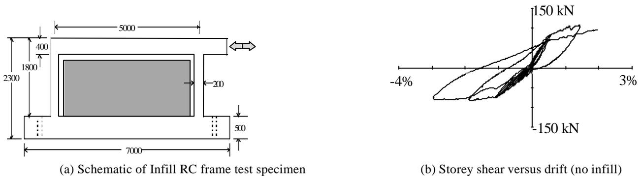
(a) Schematic of Infill RC frame test specimen
